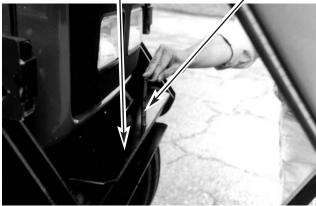
F. Loosen nut securing cuffs to loader subframe. Remove pin securing cuff. Remove cuff. (Figure 2-4)
